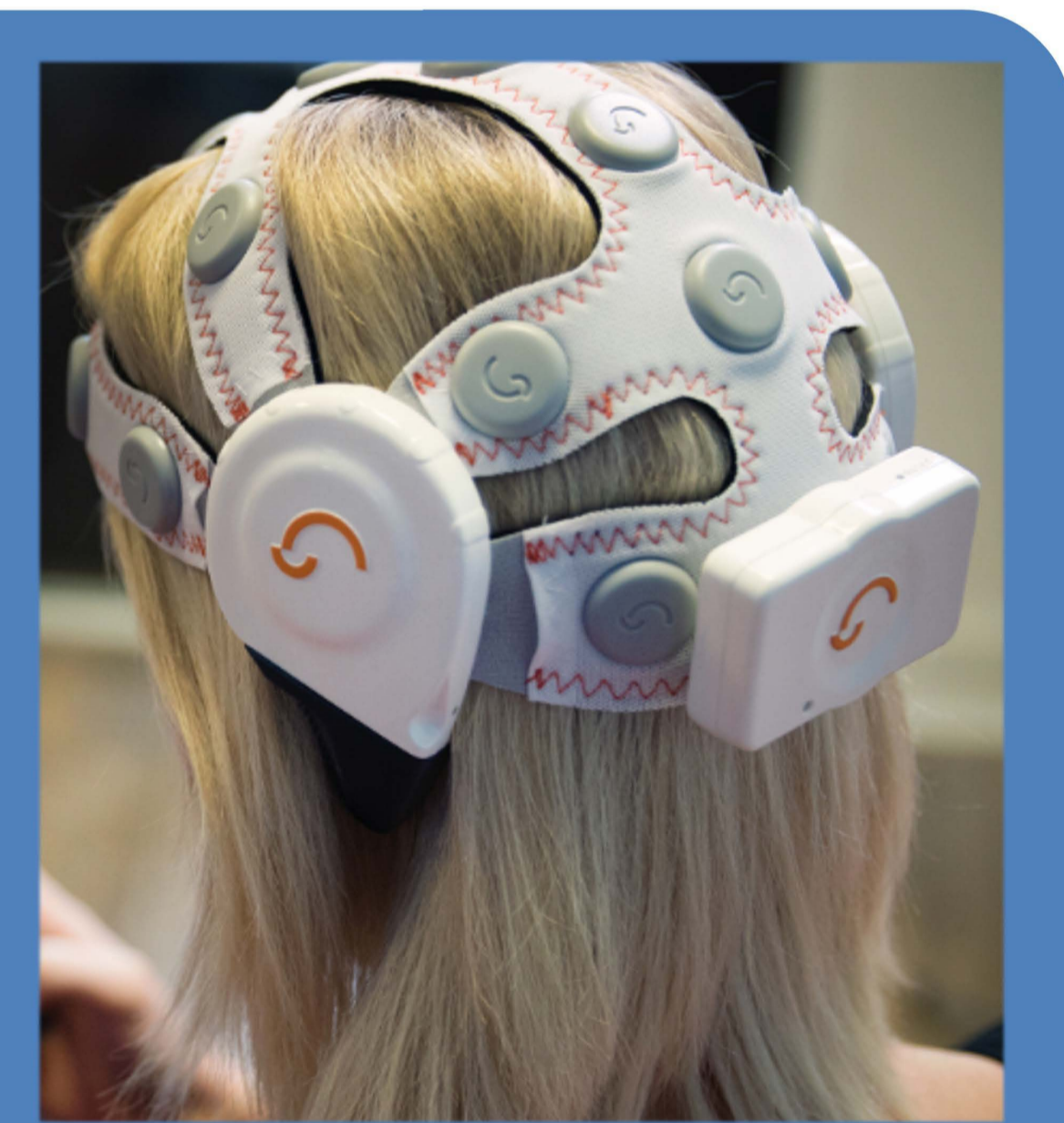
Participants were mailed a dry electrode, 16 channel, wireless EEG cap. (Cumulus, Belfast, UK).
